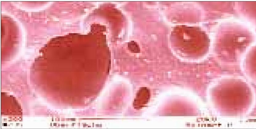
Picture of Sylomer® P, taken with a scanning electron microscope
