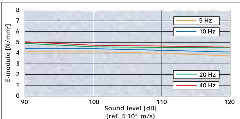
Amplitude relationship of the dynamic rigidity of Sylomer® S 600 in the usual excitation range for structural applications. Samples: 280 mm x 280 mm x 50 mm
